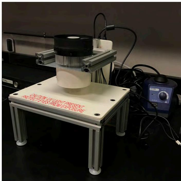
Figure 2. Dual wavelength 275 nm/405 nm LED test fixture
