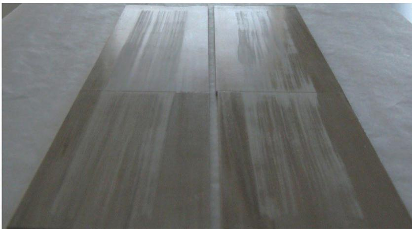
**FIGURE 7.** Showing severe scratch damage to the “control” formulation when cured using LED/UV under air due to insufficient cure after 8 passes through 385nm and 365nm LED arrays
