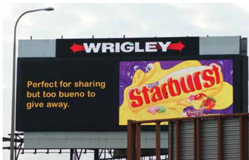
Message-changing highway billboard with red, green and blue high-brightness LEDs.
