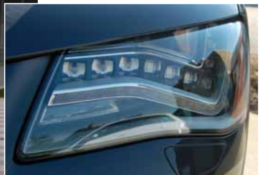
High-brightness Formula One rain tail light (left) and high-brightness headlight (above) are examples of common high-brightness LED applications.
