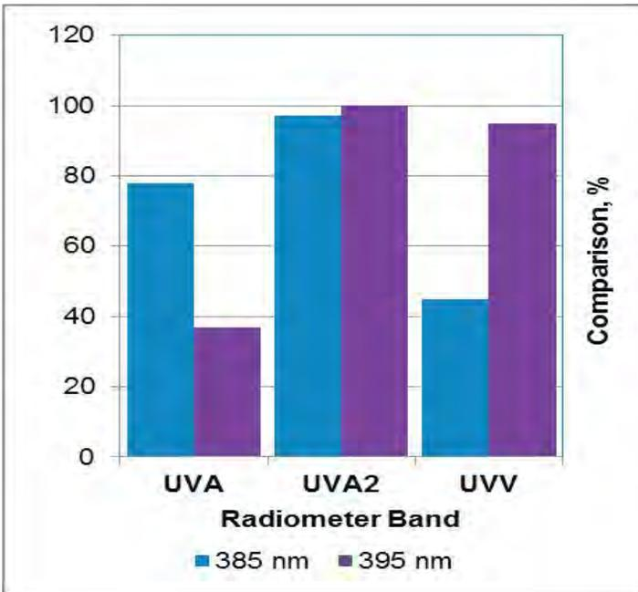
**FIGURE 6.** Measurement error related to using the wrong (UVA or UVV) measurement band with 385 nm or 395 nm LEDs
