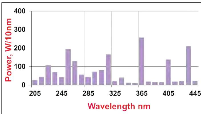
**FIGURE 3.** Spectral distribution of MP mercury UV source (shown in 10 nm integration)
