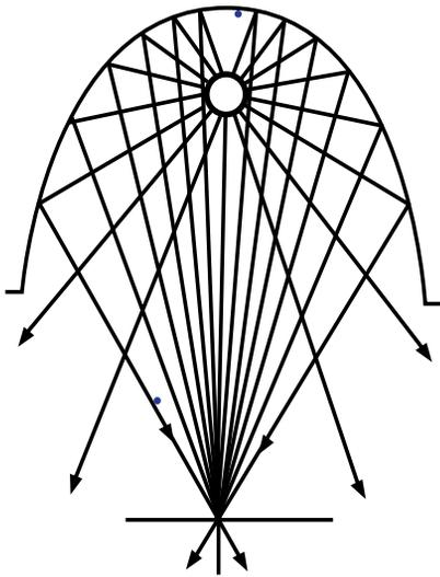
**FIGURE 1.** Typical elliptical “focusing” reflector used with MP UV lamps
