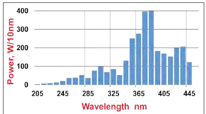
**FIGURE 4.** Spectral distribution of MP mercury UV source with iron halide additive to enhance the UVA band (“D” bulb)
