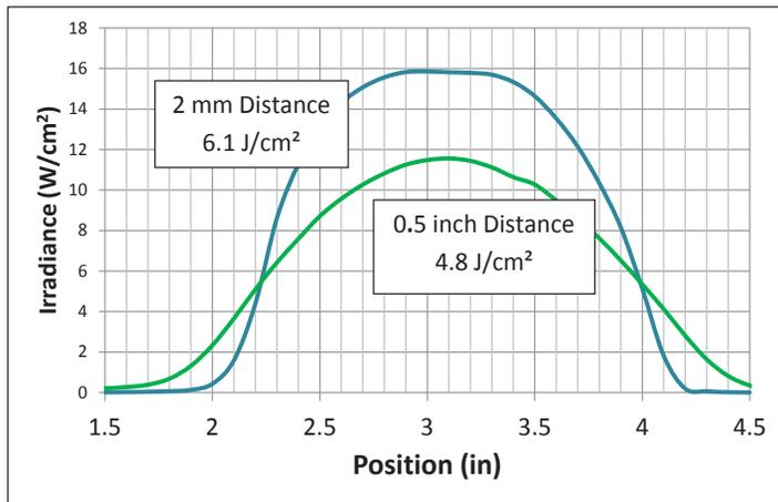
**FIGURE 7.** Irradiance profiles of 16 W/cm<sup>2</sup> 385-nm LED at 2 mm and 0.50 in. from lamp face (UVA2 exposure at 20 fpm)
