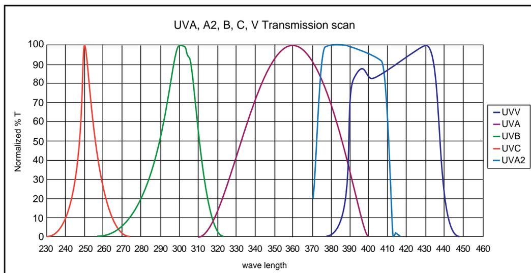
**FIGURE 5.** Several measurement bands used for MP-UV lamps and UVA2 band for UV-LEDs (Courtesy of EIT)
