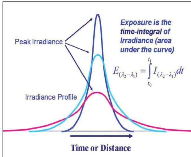
**FIGURE 2.** Typical irradiance profiles of MP UV lamps
